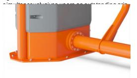
The input shaft is Ø101,3 x 2,9mm S355 Hot Dip Galvanized and Powder-coated steel. The bearing house is Caste Aluminum (EN AB-44100 / EN AB-AlSi12(a)) with self-aligning sealed ball bearings. An extremely strong and durable construction
