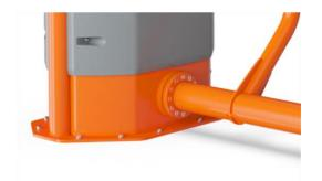
The input shaft is Ø101,3 x 2,9mm S355 Hot Dip Galvanized and Powder-coated steel. The bearing house is Caste Aluminum (EN AB-44100/EN AB-AISi12(a)) with self-aligning sealed ball bearings. An extremely strong and durable construction
