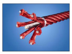
Corocord ropes with 19mm diameter or more are special 'Hercules' - type with galvanised sixstranded steel wires. Each strand is tightly wrapped with PES yarn, which is melted onto each indivudual strand. The ropes are highly wear-and vandalism-resistant and can be replaced at site if needed.
