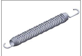
All 72 springs are made of stainless steel to ensure durability and excellent corrosion resistance. The steel wire is 3,2 mm thick and the last five windings are cone shaped to ensure long lifetime of the jumper.
